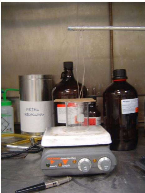
Figure 2-3 Photograph of the saturation station. Membranes were exposed to 100% relative humidity condition in this saturation process.
